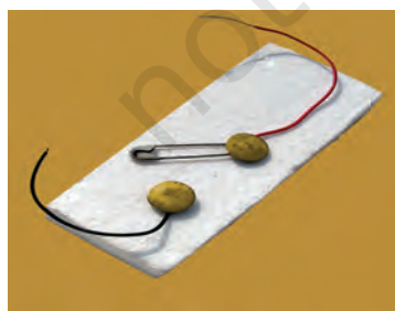
Fig. 9.8 A simple switch
