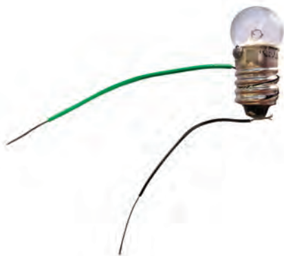
Fig. 9.4 Bulb connected to two wires
